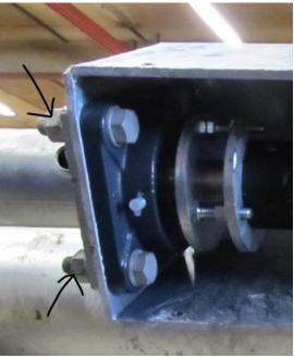
Take out the breaker bolt that secures the drive shaft to the double joint. Loosen set screws on the bearing.
