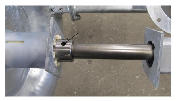
Remove the impeller from the drive shaft.
