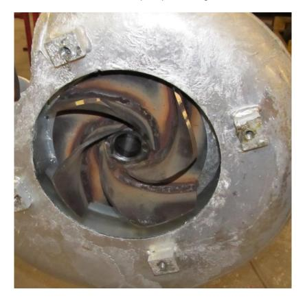
Pull out the drive shaft and impeller together. Check for runout in the drive shaft. If there is runout in the shaft, take out the breaker bolt that secures the impeller to the drive shaft.
