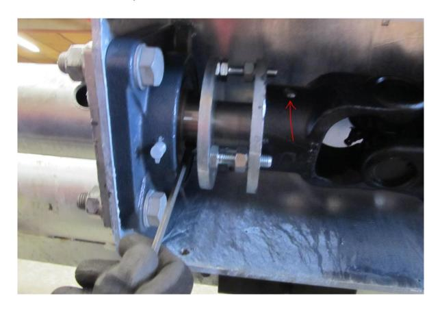
Release the cutter on the pump housing.
