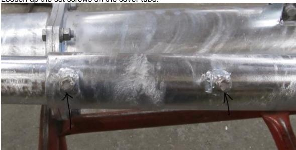
Release the cover tube at both ends. Then the bearing will also come loose.
